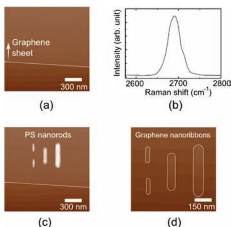
**Figure 2.** (a) Atomic force microscopy (AFM) image of the graphene sheet on the SrTiO<sub>3</sub> substrate. (b) Raman spectroscopy of the graphene sheet in (a). (c) AFM image of the graphene sheet with the PS nanorods. (d) AFM image of various graphene nanoribbons on the substrate. The white dotted lines indicate the graphene boundary.
