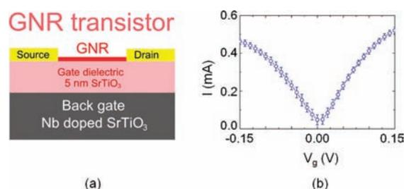
**Figure 4.** (a) Schematic side view of a GNR FET where the GNR channel is connected to the source and drain. Here, the SrTiO<sub>3</sub> substrate and Nb-doped SrTiO<sub>3</sub> substrate are used as an insulating layer and a back gate, respectively. (b) Performance of the GNR FET with an error bar as a function of the applied gate voltage  $V_g$ , where  $I$  is the source–drain current.
