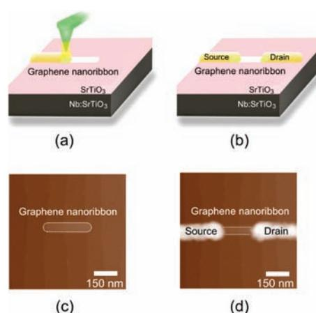
**Figure 3.** A graphene nanoribbon (GNR) field effect transistor (FET). (a) A DPN tip deposits a Au electrode as a source. (b) Schematic of the GNR FET composed of a GNR channel, an adjacent source and drain, and a back gate (Nb-doped SrTiO<sub>3</sub> substrate) after the DPN processes. AFM images of (c) only a GNR and (d) the GNR FET labeled with sample A. The white dotted lines indicate the graphene boundary.
