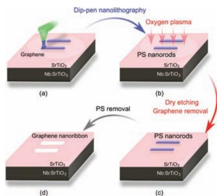
**Figure 1.** Schematic of the polystyrene (PS) dip-pen nanolithography (DPN) method. (a) A DPN tip writes PS nanorods onto a graphene sheet on a SrTiO<sub>3</sub>/Nb-doped SrTiO<sub>3</sub> substrate. (b) Oxygen plasma etches the graphene sheet with the PS nanorods on the substrate. (c) Only PS nanorods remain on the substrate. (d) Graphene nanoribbons are formed after removing the PS nanorods.
